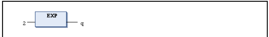
Fig.5-136: Operator EXP in FBD Operator EXP in ST
